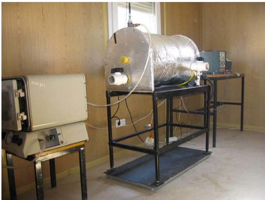
HSAD anaerobic bioreactor
